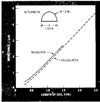
3. Microhenries. Inductance of ribbon-cable inductor is shown as a function of coil length. I. Since ribbon has 10 conductors per inch of width (coil length), abscissa represents 0 to 25 turns.
